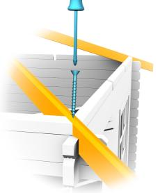
INSTALL THE ROOF PURLINS (RFB) AND ATTACH THEM WITH SCREWS.
